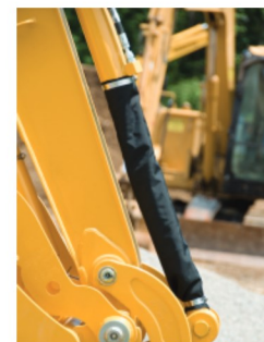
DWN is perfect for protecting hydraulic pistons in harsh environments.
