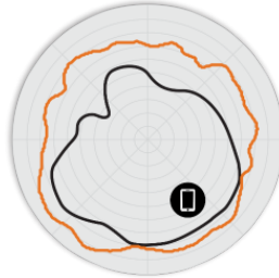
Figure 6. R770 5GHz Elevation Antenna Patterns
