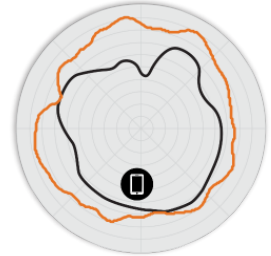
Figure 7. R770 6GHz Elevation Antenna Patterns
