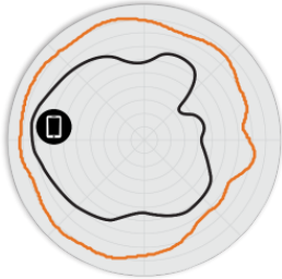
Figure 5. R770 2.4GHz Elevation Antenna Patterns
