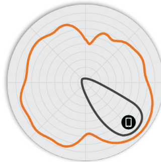
Figure 4. R550 2.4GHz Elevation Antenna Patterns
