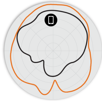
Figure 3. H550 5GHz Azimuth Antenna Patterns
