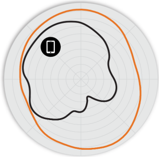
Figure 2. H550 2.4GHz Azimuth Antenna Patterns
